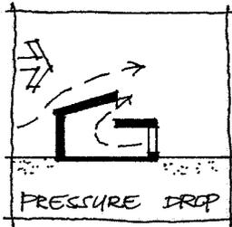
Air flowing over an obstacle, including buildings, will modify in flow speed and air pressure relative to various parts of the obstacle's surface. Broadly, air pressure at upwind surfaces will be higher than ambient pressure while sheltered or leeward places will be at lower pressure.
