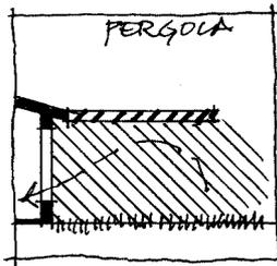
Passive solar design advocates the pergola as a shading device on the northern building side to reduce heat load on the building. The climate responsive approach uses the pergola as a design element on the southern, shade side of the building to enhance the cool characteristics of the air volume there. This cooler air is then available to be drawn into the building during the day.
