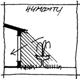
Adding moisture to ambient air in arid locations both increases its mass and its latent heat capacity. This is the basis of all evaporative air conditioning. However, systems using natural means take advantage of the tendency of humidified air to sink to ground level, to 'lean' against ambient air and press it aside.
