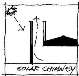
The system in the US is called a 'cool tower'. The Thompson and Cunningham trial in Phoenix also included windcatcher elements at the top of the tower, and a solar heat chimney exhaust at the other end of the building. Givoni (1994) considered the tower airflow both in its role in occupant space ventilation, and ventilation within the building fabric to extract heat from the building structure.
