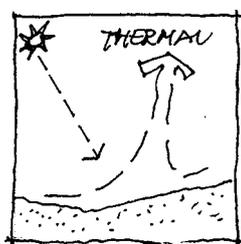
Air in external spaces solar heated to temperatures higher than ambient results in an expanding air volume, which is lower in air density than the surrounding ambient air. This imbalance is solved by thermal convection. The lighter air streams upward either as a bubble or a funnel shaped column, being replaced by ground level horizontal air inflow which in turn is heated and the process repeats.
