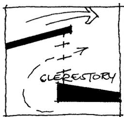
Such building form also provides opportunities for openings at the low pressure portion of the building roof shape in relation to summer winds. Thereby air from the occupied spaces can be drawn outward as a deliberate secondary airstream using the roof top suction from northerly winds which are otherwise unusable, being hot, dry and embedded with dust.
