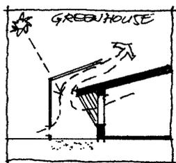
The traditional greenhouse is a solar heated space either for comfort in cool climates, or for enhanced propagation of vegetation, notably that not native to the location.
