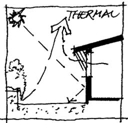
Ground adjacent to a northerly face of a building is subject to solar heat load both from direct sunlight, and reflected heat from adjacent surfaces, notably the building exterior itself. The air in this location reaches temperatures higher than ambient, and vents vertically by thermal convection. From this pressure reduction at ground level, suction draws ground level air in from all around, including through abutting openings in the adjacent building itself.
