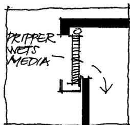
In the US, material used for the filter pad is cardboard egg-crate matrix 'CELdek', whereas local installations to date have used 'Woodwool' media. Both are standard evaporative air conditioner materials. 'Woodwool' consists of aspen shavings which fully wet up. This
