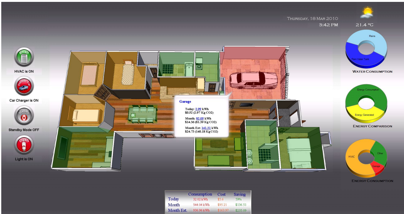
The energy management screen shows residents at a glance their energy consumption throughout the house (Image courtesy of La Trobe University)
