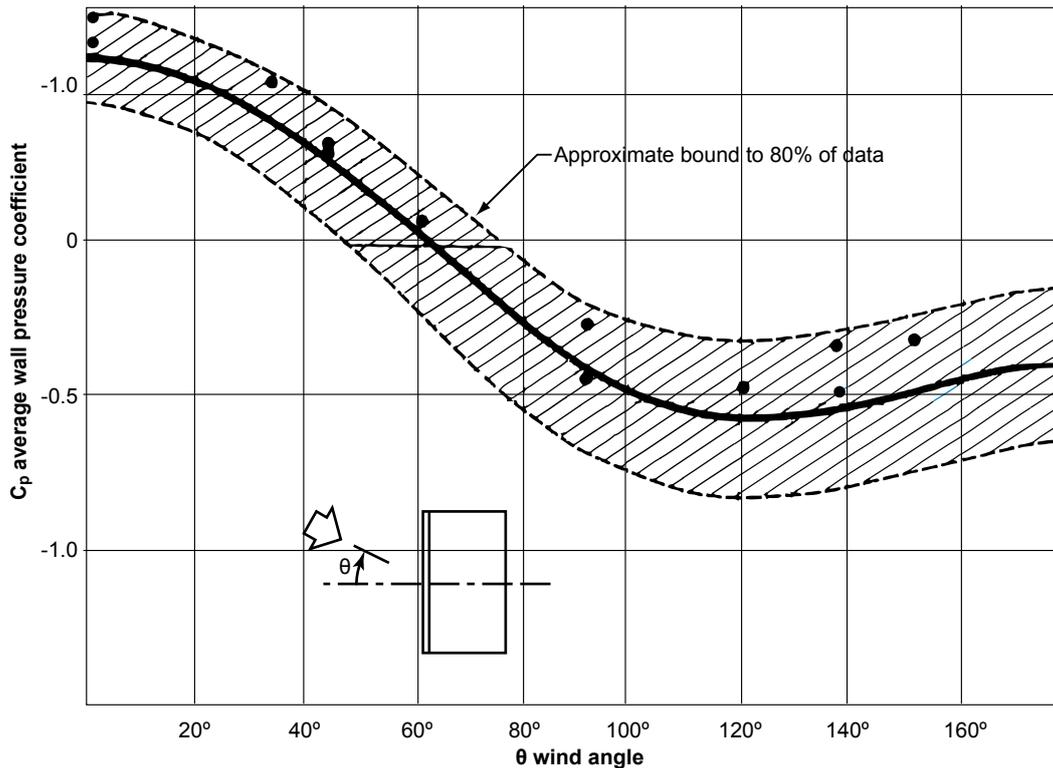
**Figure 3. Typical Wall-averaged Wind pressure Coefficients for Low-rise Buildings**
