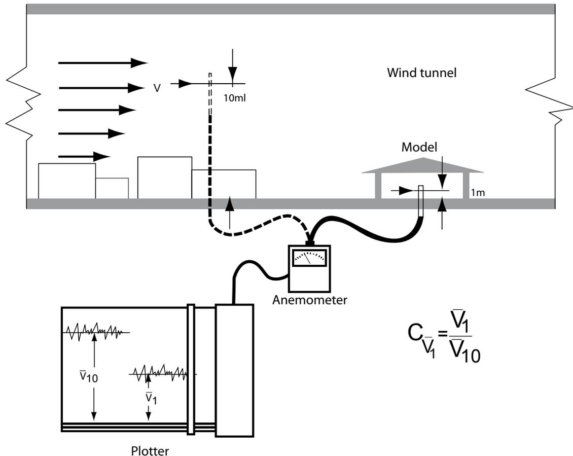
Figure 5. Indoor wind speed coefficient measurement in a boundary layer wind tunnel
